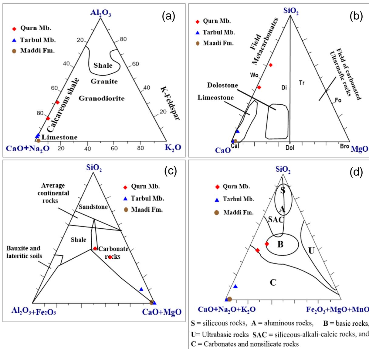
Fig. 7 (a). Ternary diagram (Hutcheon, 1998) between  $Al_2O_3$  -  $(CaO+Na_2O)$  -  $(K_2O)$  for the studied samples, (b) Ternary diagram between  $SiO_2$  -  $CaO$  -  $(MgO)$  (Winter, 2001) for the studied samples, (c) Ternary diagram between  $SiO_2$  -  $(Al_2O_3+Fe_2O_3)$  -  $(CaO+MgO)$  (Mason & Moor, 1982) for the studied samples, and (d) Ternary diagram between  $SiO_2$  -  $(CaO+Na_2O+K_2O)$  -  $(Fe_2O_3+MgO+MnO)$  (Raymond, 1995) for the studied samples.
