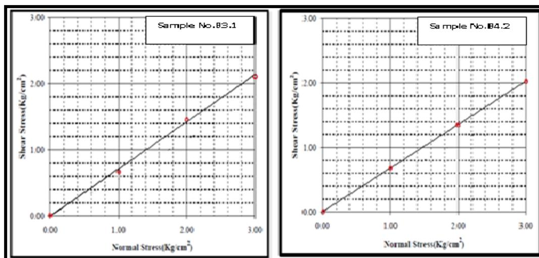
Fig. 4. Normal stress and shear stress of some samples.
