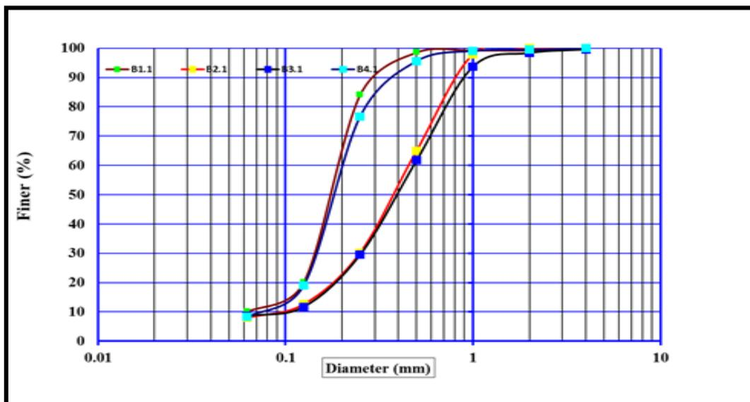
**Fig. 2. Distribution curve of some samples.**
