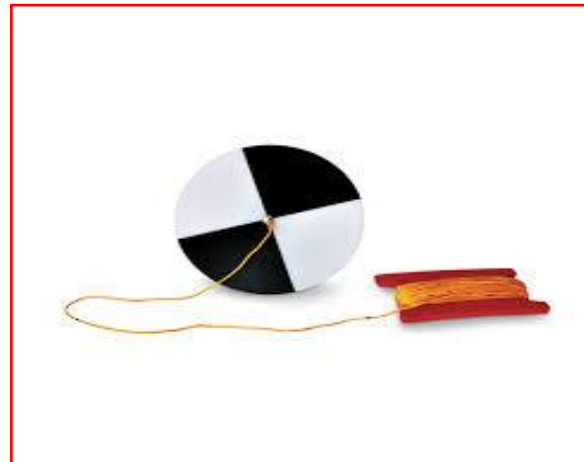
Fig. 3. Shows white/black Secchi Disk, water testing (20 cm in diameter).
