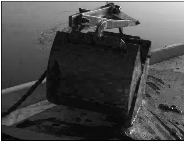
Fig. 2. shows Ekman dredge bottom sampler.
