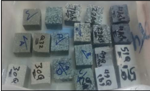
Fig. 5: Photograph showing the studied specimens (granite, rhyolite and marble) immersed by tap water at 20 \pm 10^\circ\text{C} Cup half the height of the specimens.
