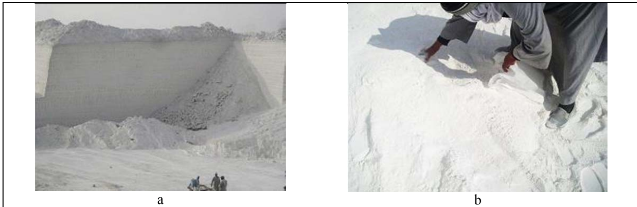
Fig. 1: Field photos for a quarry of pure limestone at El Minia, East Nile Valley, (a) Large limestone outcrop (b) Calcium carbonate powder (5-20um)
